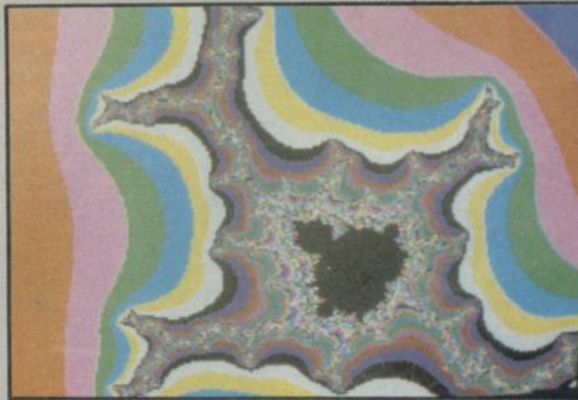
Coupe screen in Mode 4 – The graphics mode with 256 x 192. 16 colours from a palette of 64 at any pixel.
